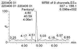
Figure 7: Chromatogram - LC-MS/MS Analysis - Sample
