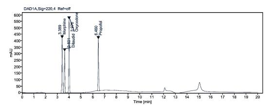
Figure 3: Chromatogram – HPLC Analysis – High Standard (S6)
