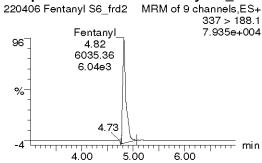
Figure 6: Chromatogram - LC-MS/MS Analysis - High Standard (S6)
