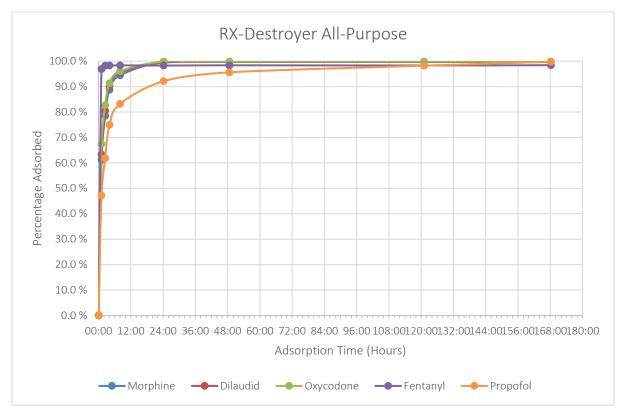
Figure 13: Adsorption of API's vs Contact Time
