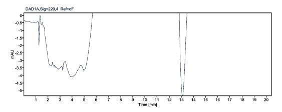
Figure 2: Chromatogram – HPLC Analysis – Blank (S0)
