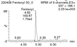
Figure 5: Chromatogram - LC-MS/MS Analysis - Blank (S0)
