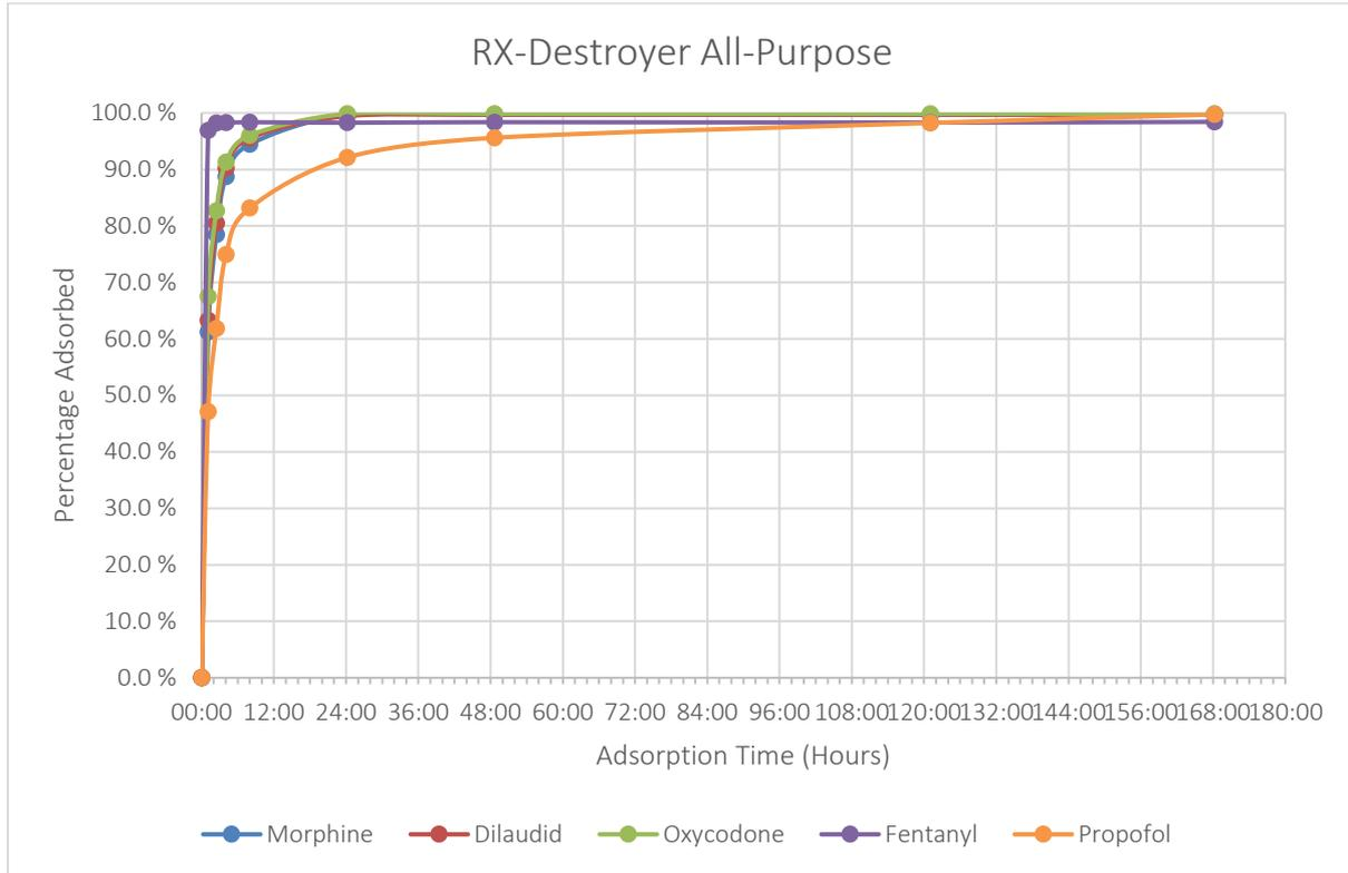
Figure 13: Adsorption of API's vs Contact Time
