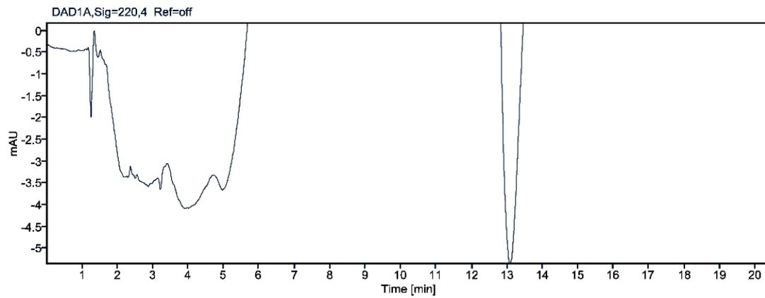
Figure 16: HPLC Chromatogram - Calibration Standard 1
